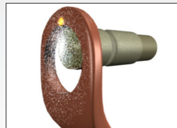
3 The capsule of the brazing pin opens. A special flux powder cleans the surface.
