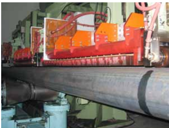
A detail from an EFD Induction seam normalizing solution. The induction coils are the red horizontal units above the pipe.
