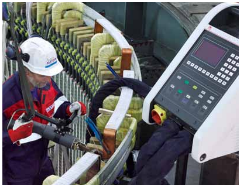
An EFD Induction Minac brazes generator windings. Minac's mobility and the handheld transformer let operators access hard-to-reach areas.
