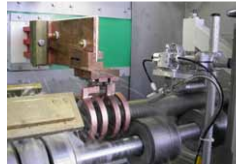
A shaft moving at high speed through an induction coil. Induction tempering is unrivalled for its speed and precision.
