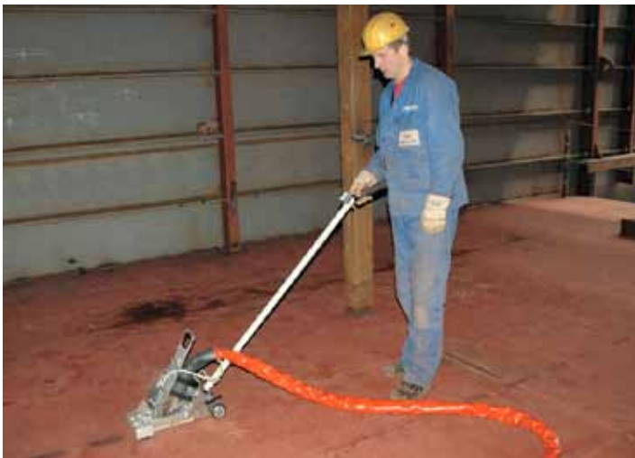
An EFD Induction Terac system ensures failsafe operation—it makes it impossible to overheat magnetic steel. Moreover, Terac does not produce toxic gases from the heating source. And there is no acoustic noise.
