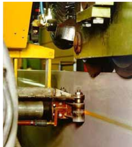
The benefits of induction straightening are not limited to the shipbuilding industry. Here, an EFD Induction system straightens T-beams for a construction project.
