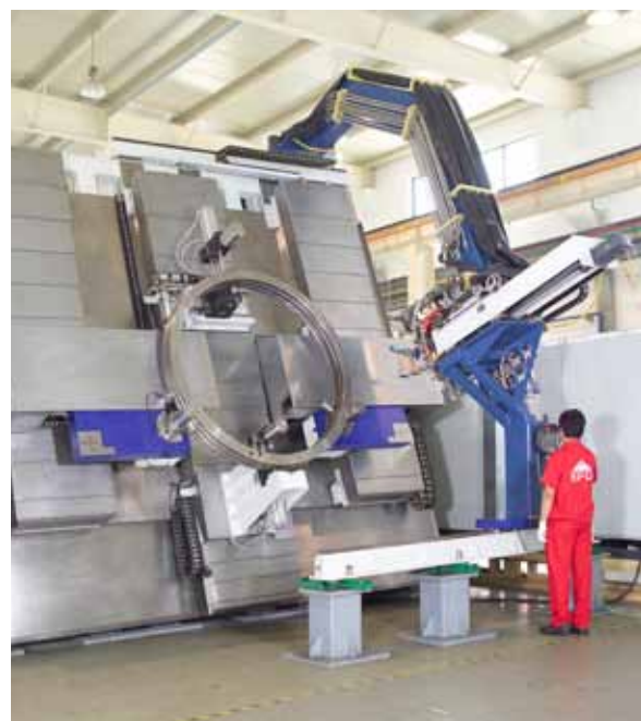
A large ring being hardened by an EFD Induction vertical scanning hardening machine.
