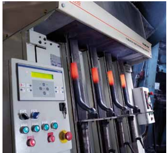
Above, an EFD Induction vertical partial heater. These systems can be fitted with any number of induction coils, and are available in IGBT and thyristor versions.
