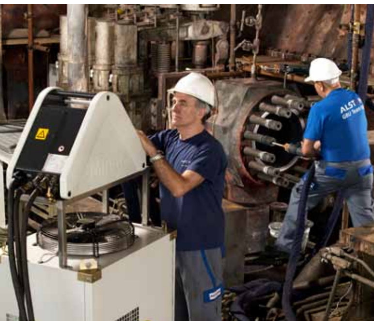
An example of shrink fitting—EFD Induction equipment removes large nuts and bolts in a fraction of the time needed by traditional gas or resistance heating.
