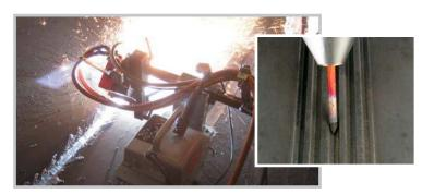
The Arcair-Matic® N7500 gouging system is highly productive for any metal fabrication operation where gouging and welding represents a large portion of the work schedule. This applies to almost all metals, including stainless steel, carbon, manganese, and chrome-moly steels.
